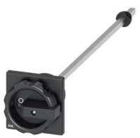
Door-coupling rotary operating mechanism black 66x66 mm, Front plate mounting Central hole mounting 22.5mm with coupling part with shaft 300 mm long, 6x6 mm, accessories for load disconnector 3LD3
